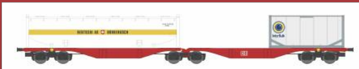
Carro intermodale articolato Tipo Sggrss 80' DB con carico di silos e tank container. Articulated container wagon Type Sggrss 80' of DB with silos and tank container. Gelenk-Containertragwagen Typ Sggrss 80' der DB mit Silos und Tank Container.
