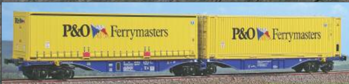
Carro intermodale Tipo Sggmrss '90 bimodulo noleggiato "P&O Ferrymasters" carico di casse mobili. Container wagon Type Sggmrss '90 hired by "P&O Ferrymasters" with swap bodies. Containerwagen Typ Sggmrss '90 Doppelmodul vermietet an "P&O Ferrymasters" mit Wechselpritschen.
