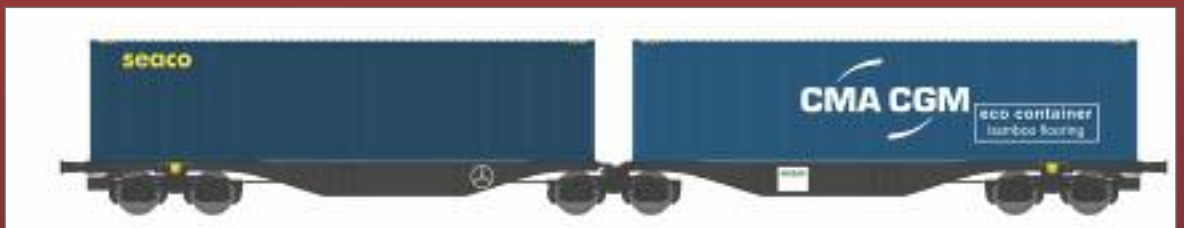
Carro intermodale articolato Tipo Sggrss 80' Adria Kombi con carico di container. Articulated container wagon Type Sggrss 80' of Adria Kombi with container. Gelenk-Containertragwagen Typ Sggrss 80' der Adria Kombi mit Containern.
