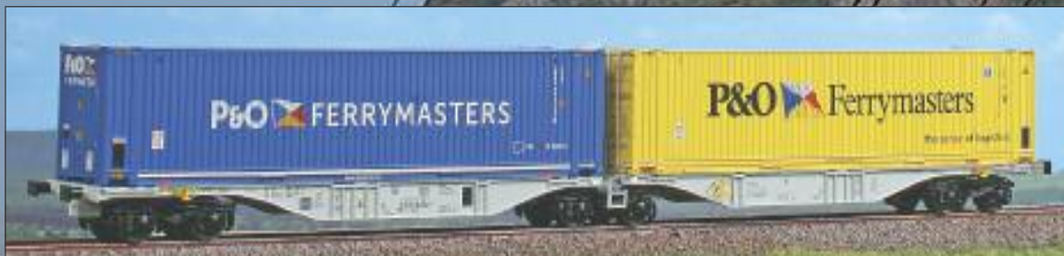
Carro intermodale Tipo Sggmrss '90 bimodulo noleggiato "P&O Ferrymasters" carico di casse mobili. Container wagon Type Sggmrss '90 hired by "P&O Ferrymasters" with swap bodies. Containerwagen Typ Sggmrss '90 Doppelmodul vermietet an "P&O Ferrymasters" mit Wechselpritschen.
