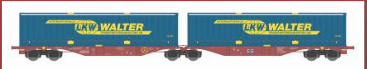
Carro intermodale articolato Tipo Sggmrss 90' Touax noleggiato "CEMAT" con carico di casse mobili. Articulated container wagon Type Sggmrss 90' Touax hired by "CEMAT" with swap bodies. Gelenk-Containertragwagen Typ Sggmrss 90' Touax an "CEMAT" vermietet mit Wechselpritschen.
