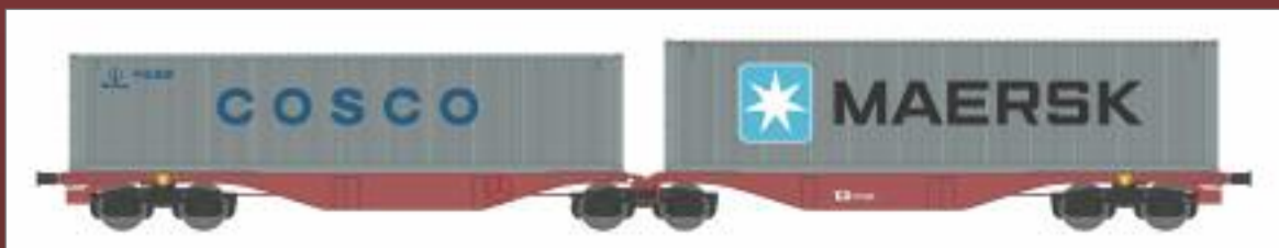
Carro intermodale articolato Tipo Sggrss 80' ĆD Cargo con carico di container. Articulated container wagon Type Sggrss 80' of ĆD Cargo with container. Gelenk-Containertragwagen Typ Sggrss 80' der ĆD Cargo mit Containern.
