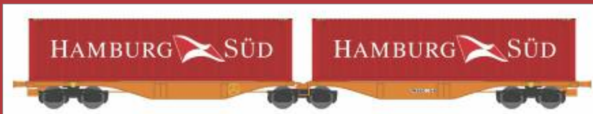
Carro intermodale articolato Tipo Sggrss 80' WASCOSA con carico di container. Articulated container wagon Type Sggrss 80' of WASCOSA with container. Gelenk-Containertragwagen Typ Sggrss 80' der WASCOSA mit Containern.
