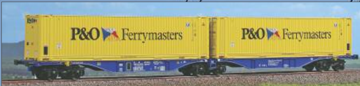
Carro intermodale Tipo Sggmrss '90 bimodulo noleggiato "P&O Ferrymasters" carico di casse mobili. Container wagon Type Sggmrss '90 hired by "P&O Ferrymasters" with swap bodies. Containerwagen Typ Sggmrss '90 Doppelmodul vermietet an "P&O Ferrymasters" mit Wechselpritschen.
