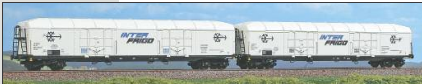
Set di due carri isothermici a carrelli INTERFRIGO, immatricolati FS, con logo moderno. Set of two INTERFRIGO isothermic wagons, with bogies, registered at the FS, with modern logo. Set aus zwei isothermischen INTERFRIGO-Drehgestell-Wagen, bei der FS eingestellt, mit modernem logo.
