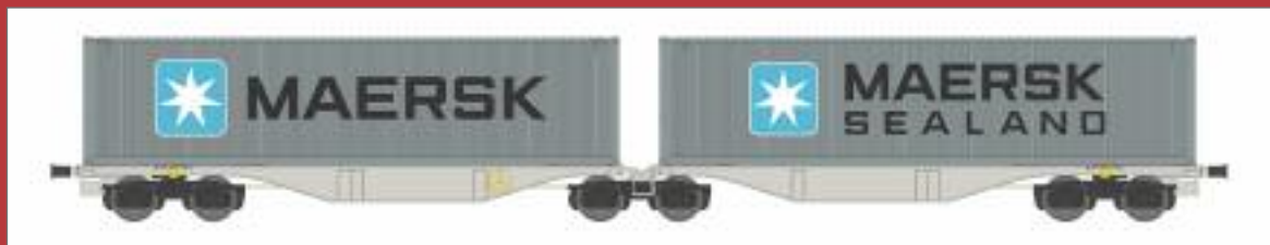
Carro intermodale articolato Tipo Sggrss 80' AAE con carico di container. Articulated container wagon Type Sggrss 80' of AAE with container. Gelenk-Containertragwagen Typ Sggrss 80' der AAE mit Containern.
